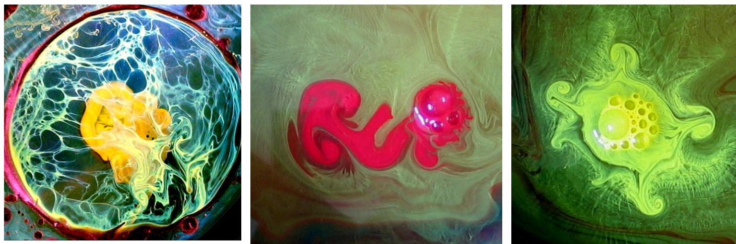
Fig. 6. Some developing vortices. The radial spread on the left has its original vortices as well as a well-developed network, whose 3-dimensional aspect is apparent. The other two images also have bubbles marking the stagnation point.
